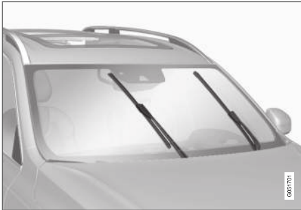
Viskerblader i servicestilling.
