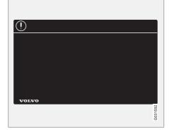
White ISO symbols on black symbol field, white text/image on black message field. If a colour is required then the decal shall be blue. Dangerous situation which, if not avoided, may result in minor or moderate damage to property.
