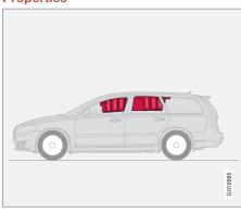
The inflatable curtain IC (Inflatable Curtain) is a supplement to the SIPS and the airbags. It is fitted in the headlining along both sides of the roof and protects all of the vehicle's outer seats. A sufficiently violent collision trips the sensors and the inflatable curtain is inflated. The inflatable curtain helps to prevent the driver and passengers from striking their heads on the inside of the car during a collision.
