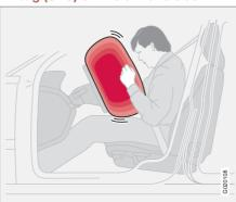
The car has an SRS airbag (Supplemental Restraint System) in the steering wheel to supplement the protection afforded by the seatbelt on the driver's side. This airbag is folded up into the centre of the steering wheel. The steering wheel is marked **SRS AIRBAG**.
