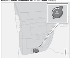
The electrical socket can be used for various accessories, such as mobile phone chargers and coolers.
