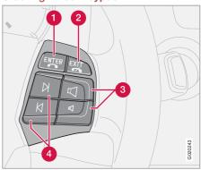
When the phone is active, the steering wheel keypad is locked to phone functions. To control the audio system, the phone must be in standby mode (standby).
