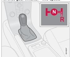
The reverse gear inhibitor hinders the possibility of mistakenly attempting to engage reverse gear during normal forward travel.
