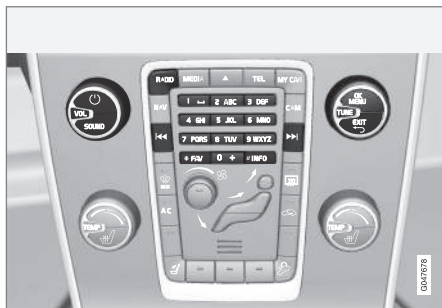
Controls for radio functions.
