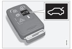
Using the remote control key (p. 160) button the alarm for the tailgate can be disarmed\* and the tailgate unlocked on its own.
