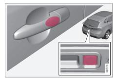
Lock the doors and the tailgate by grasping one of the door handles or pressing the smaller of the tailgate's two rubberised buttons - the lock indicator (p. 162) in the windscreen confirms that locking has been completed by starting to flash.
