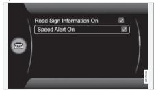
The driver can opt to receive a warning when the applicable speed limit is exceeded by 5 km/h (3 mph) or more. This warning is given by the symbol showing the applicable maximum speed temporarily flashing when this speed is exceeded.
