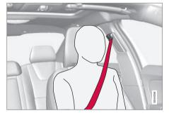
Correctly fitted seatbelt.
