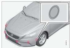
The PAP sensors are located in the bumpers<sup>39</sup> - 6 front and 4 rear.
