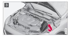
Fold the cover toward the engine to access the fuses.
