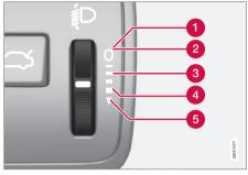
Thumbwheel positions for different load cases.
