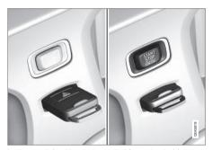
Ignition switch with remote control key extracted/inserted.
