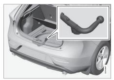
The detachable towbar must be stored in the foam block<sup>15</sup> under the cargo area floor when not in use.
