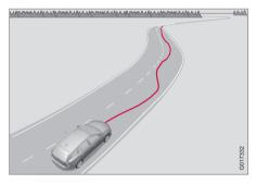
A camera detects the side markings painted on the carriageway and compares the section of the road with the driver's steering wheel movements. The driver is alerted if the vehicle does not follow the carriageway evenly.
