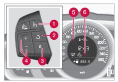
The steering wheel buttons and display in cars **with** speed limiter<sup>7</sup>.
