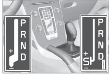
**D**: Automatic gear positions. +/-: Manual gear positions. **S**: Sport mode\*.3
