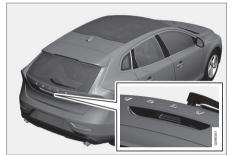
Rubber plate with electrical contact.
