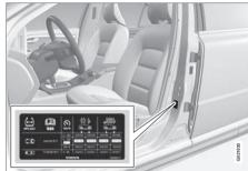
The tyre pressure label on the driver's side door pillar (between frame and rear door) shows which pressure the tyres should have at different loads and speed conditions. This is also specified in the tvre pressure table.
