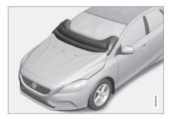
The pedestrian airbag (Pedestrian Airbag) is fitted under the bonnet near the windscreen. In the event of certain frontal collisions with a pedestrian, the sensors in the front bumper react and the airbag inflates if required, based on the force of the impact. The sensors are active at a speed of approx. 20-50 km/h (12-30 mph) and an ambient temperature between -20 and +70°C.
