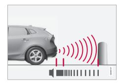
The distance covered to the rear of the car is about 1.5 metres. The acoustic signal for obstacles behind comes from one of the rear loudspeakers.
