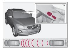
Laser sensor transmitter and receiver window<sup>15</sup>.
