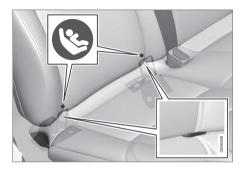
Mounting points for the ISOFIX fixture system are located at the lower section of the rear seat backrest, in the outer seats.
