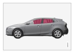
The inflatable curtain IC (Inflatable Curtain) is part of the SIPS system (p. 38). It is fitted along the headlining on both sides and helps protect the driver and passengers in the car's outer seats. A sufficiently violent collision trips the sensors and the inflatable curtain is inflated.
