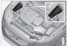
When topping up the coolant, follow the instructions on the packaging. Never top up with water only. The risk of freezing increases with both too little and too much coolant concentrate.
