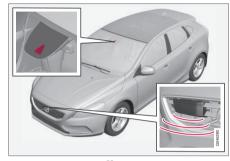
Camera and radar sensor<sup>23</sup>.
