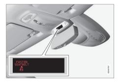
The audio reminder is speed dependent, and in some cases time dependent. The visual reminder is located in the roof console and in the combined instrument panel (p. 66).
