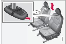
The height of the head restraints can be adjusted.
