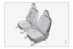
The SIPS bag system consists of two main components, side airbag and sensors. The side airbags are located in the front seat's backrests.
