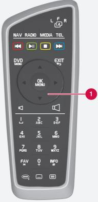
1 Scroll wheel, equivalent to TUNE in the centre console.
