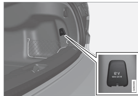
12 V electrical socket in cargo area*.
