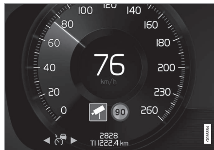
Speed camera warning in the driver display.
