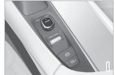
Start knob in the tunnel console.
