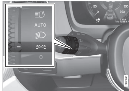
Stalk switch rotating ring in position lamps position.
