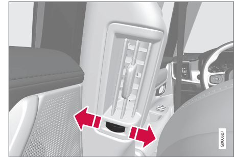
The air vent's thumbwheel 4 .
