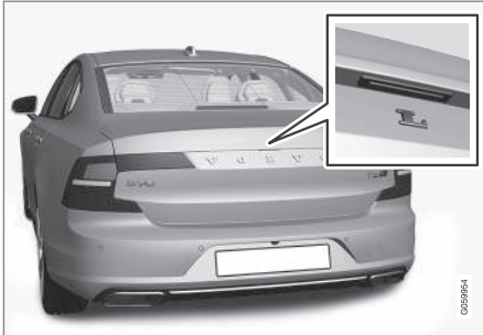
Rubber plate with pressure-sensitive surface.
