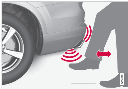
Kicking motion within the detector's valid activation area.
