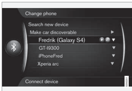
Example: a cell phone is connected as a phone and as a media player
