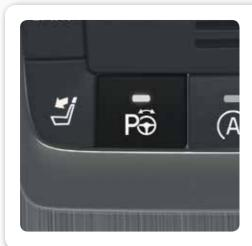
PAP determines if a parking space is big enough for your vehicle and helps to steer it into the space. The driver selects gears, regulates the vehicle's speed and applies the brakes.
