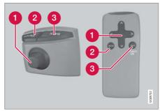
The steering wheel keypad and the keypad on the remote control have the same functions. Use the keypad to scroll through different menu options, confirm selections or move back in menus.
