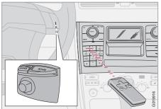
The navigation system is controlled with the steering wheel's keypad or the remote control.
