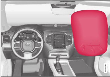
Front passenger airbag in front seat.
