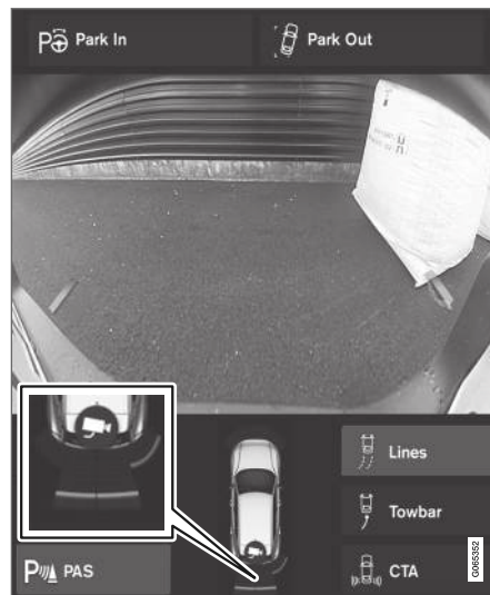
The screen can show coloured sensor fields on the car symbol 120 .
