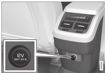
12 V electrical socket in tunnel console, second seat row.
