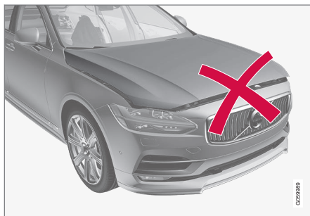
Hood not completely closed.
