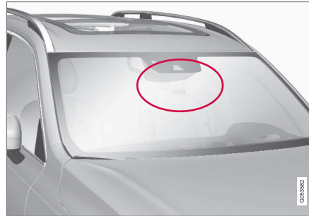
Location of radar sensor.
