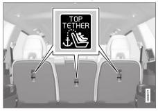
Top tether anchors and symbols on the rear side of the second row backrests. There is no symbol for the center anchor position.
