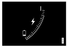
The symbol is displayed in the hybrid battery gauge when Charge is activated.
