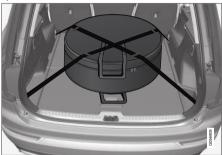
The spare wheel is stored in a bag and should be secured with two straps onto the floor of the trunk/cargo compartment when the vehicle is being driven<sup>12</sup>. The straps should be strapped down crosswise over the wheel, attached to the load anchoring eyelets and pulled taut.
