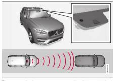
The camera/radar sensor measures the distance to the vehicle ahead42.
