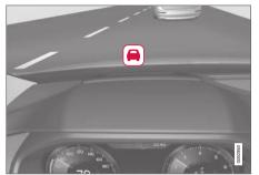
Collision warning symbol on the windshield<sup>44</sup>.
