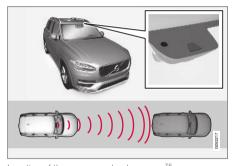
Location of the camera and radar sensor<sup>75</sup>.
