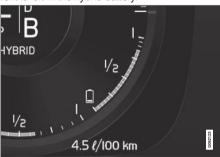
The current in the hybrid battery is used to power the electric motor, but can also be used to heat or cool the vehicle. The trip computer calculates an approximate driving distance with the remaining current in the hybrid battery.
