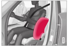
The side airbags are located in the front seats' outer backrest frames and help protect the driver and front seat passenger.
