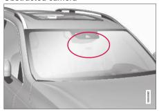
The area marked in the illustration must be kept free of decals, objects, solar film, etc.  $^{74}$
