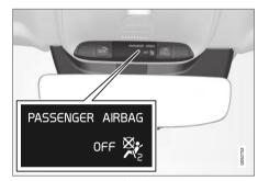
Occupant Weight Sensor (OWS) indicator light
