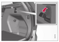
There are two fold-out holders in the side panels, one on each side of the cargo compartment.
