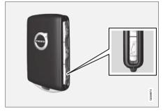
Use the button on the remote key to disarm and unlock the tailgate.
