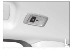
In vehicles with panoramic roofs\*, there are two lamp units, one on each side of the ceiling.7
