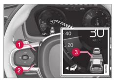
Controls for setting a time interval.
