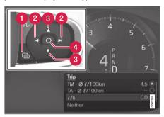
Open and navigate in the app menu using the righthand steering wheel keypad.
