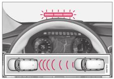
Collision warning light on the windshield<sup>43</sup>.
