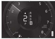
Gear indicator in instrument panel<sup>2</sup>.
