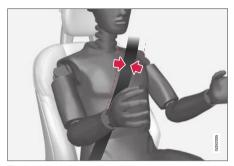
The belt should be positioned closely against the inside of the shoulder (against the collarbone, not down over the arm).
