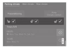
Window for seat/steering wheel heating in the **Parking** climate tab in Climate view.
