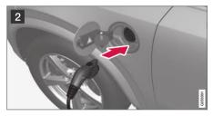
Open the charger door and remove the charging socket's protective cover. Push the charging handle all the way into the vehicle's socket.
