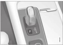
Park is activated using the **P** button located next to the gear selector.
