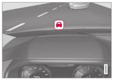
Collision warning symbol on the windshield<sup>64</sup>
