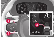
Controls for setting a time interval<sup>48</sup>.
