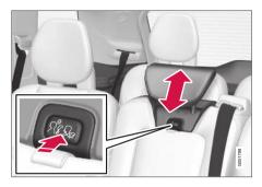
To lower the restraint, press and hold the button (located between the backrest and the head restraint, see illustration) while carefully lowering the head restraint.
