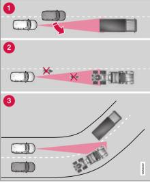
The radar sensor's field of vision.
