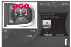
Messages in the instrument panel and the right-side steering wheel keypad.
