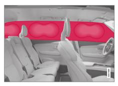
The inflatable curtains are installed along both sides of the inside of the roof and help protect occupants in the vehicle's outer seats. **IC AIRBAG** is embossed on the panels.
