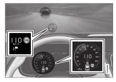
The previous illustration<sup>61</sup> shows that Adaptive Cruise Control is set to maintain a speed of 110 km/h (68 mph) and is following a target
