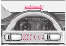
Collision warning light on the windshield<sup>63</sup>.
