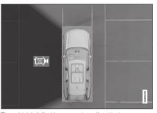
The vehicle's left-side camera is malfunctioning.
