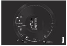
The vehicle generates electrical current to charge the battery, e.g. when the driver lightly presses the brake pedal or when engine braking is used on downgrades.
