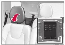
The outer head restraints can be folded via the center display's function view. The head restraint can be folded down when the vehicle is in ignition mode **0**.
