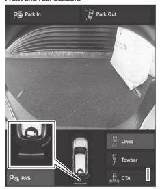
The screen can display colored sensor fields on the vehicle symbol <sup>122</sup>.
