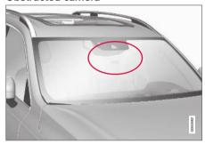
The area marked in the illustration must be kept free of decals, objects, solar film, etc. 70
