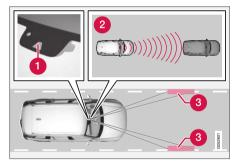
The camera/radar sensor monitors the distance to the vehicle ahead and detects lane markings<sup>62</sup>.
