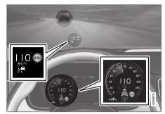
The previous illustration<sup>69</sup> shows that Pilot Assist is set to maintain a speed of 110 km/h (68 mph) and is following a target vehicle ahead that is traveling at the same speed.
