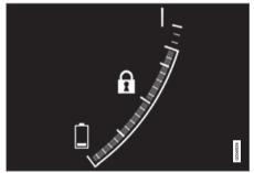
The symbol is displayed in the hybrid battery gauge when Hold is activated.
