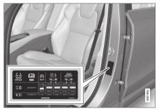
The placard specifies the designation for the factory-mounted tires on the vehicle, as well as load limits and inflation pressures.
