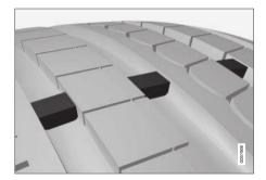
The tread wear indicator is a narrow elevated strip running across the tire's longitudinal tread grooves. The letters TWI (Tread Wear Indicator) are visible on the side of the tire. When approximately 1.6 mm (1/16 inch) is left on the tread, the tread will be at the same height as the tread wear indicator. Replace the tire as soon as possible. Tires with low tread offer very poor traction in rain or snow.
