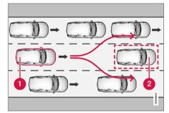
Your vehicle (1) cannot detect any potential escape routes for veering away from the vehicle ahead (2) and may therefore apply the brakes at an earlier stage.
