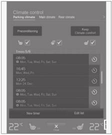
Preconditioning and the climate comfort retaining function are controlled from the **Parking climate** tab in the center display's Climate view.
