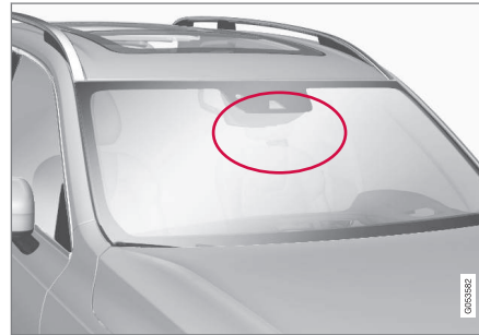
Radar unit location.
