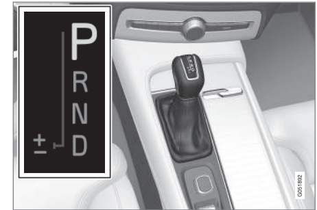
Overview of large gear lever and shift pattern in the driver display.
