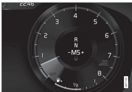
Driver display when changing gear with steering wheel paddles in manual gearshift mode, small gear lever.
