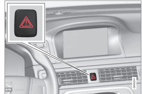
Button for hazard warning flashers.
