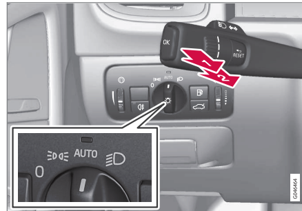
Stalk switch and knob for headlamp control.
