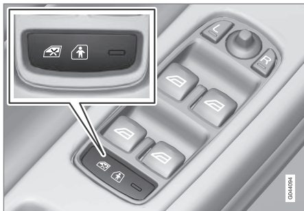
Control panel driver's door.
