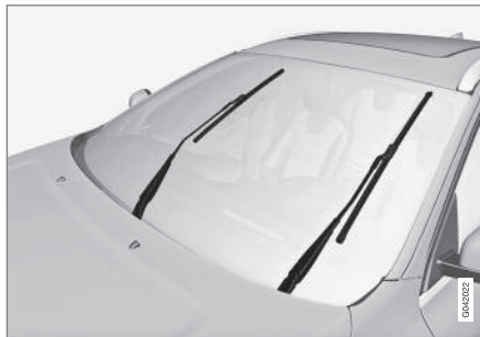
Wiper blades in service position.
