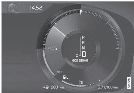
Eco gauge in the 12-inch driver display.
