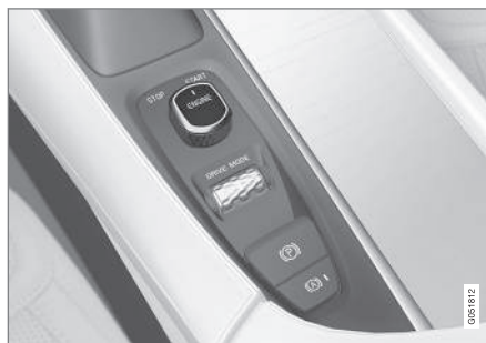
Start knob in the tunnel console.
