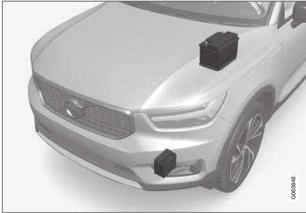
The support battery is located in the engine compartment. The start battery is also shown here (top).
