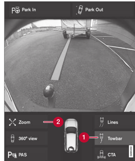
Towbar with trajectory line.
