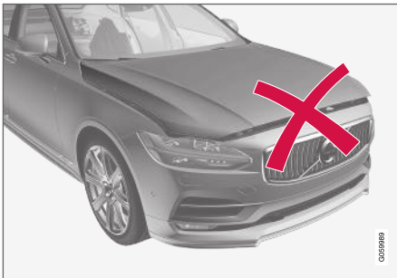
Hood not completely closed.
