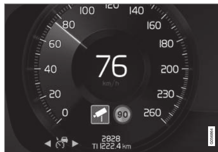
Speed camera information in the instrument panel.
