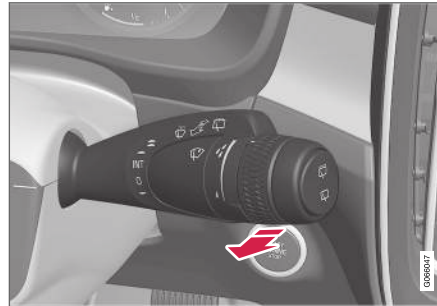
Washing function, right-hand steering wheel lever.
