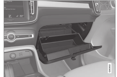
Glove compartment with fold-out hook.
