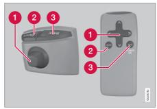
The steering wheel keypad and the keypad on the remote control have the same functions. Use it to scroll between different menu options, to confirm selections or to move back in menus.
