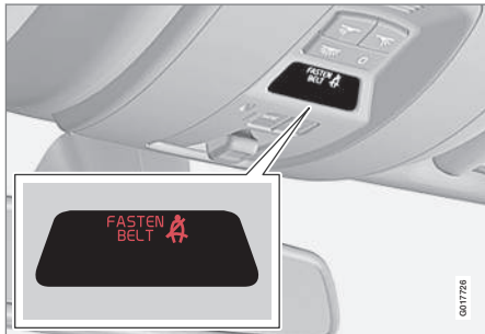
Seat belt reminder light in ceiling console
