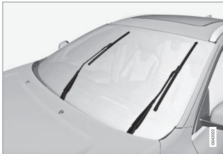
Wiper blades in service position
