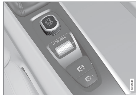
Start knob in the tunnel console.
