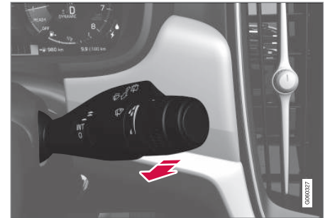
Washing function, right-hand steering wheel lever.
