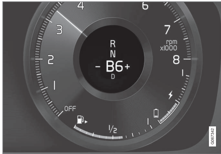
Brake position in instrument panel overview.
