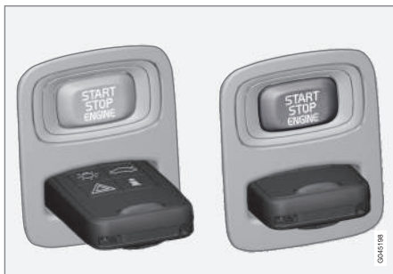
Ignition switch with remote control key extracted/inserted.
