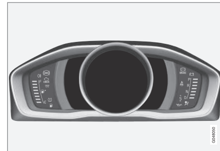
Information display, digital instrument panel*.
