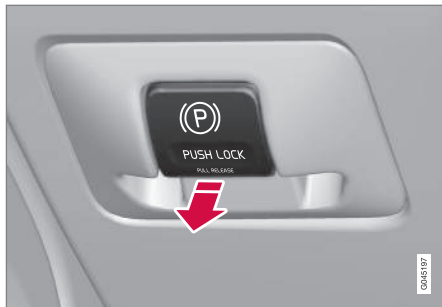
Parking brake control - release.
