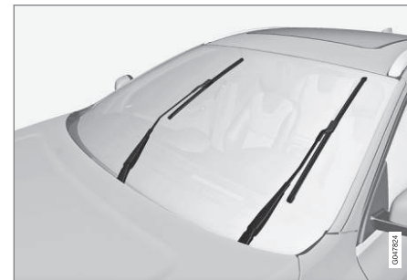
Wiper blades in service position.
