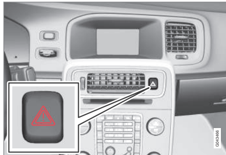
Button for hazard warning flashers.
