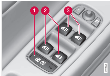
Driver's door control panel.
