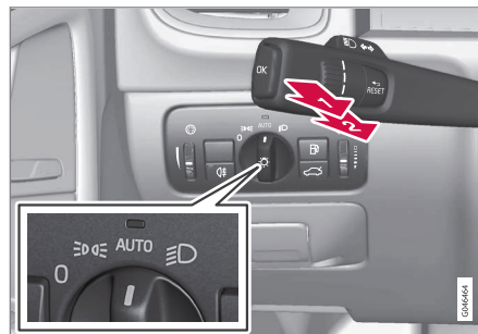
Stalk switch and knob for headlamp control.
