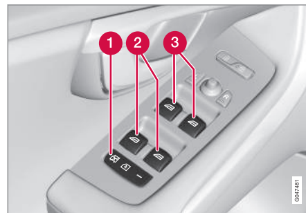
Driver's door control panel.
