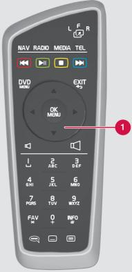
Scroll wheel, equivalent to **TUNE** in the centre console.
