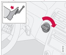
Keyless drive makes it possible to unlock, start and lock the vehicle without using a remote key.
