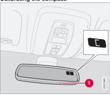
The earth is divided into 15 magnetic zones. The compass is initially set for the zone to which the car was delivered, and should always be adjusted if the car is driven to a new magnetic zone. A "C" will be displayed if calibration becomes necessary.
