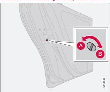
The controls are located on the rear inside edges of the doors, and are only accessible when the doors are open.
