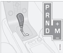
**D** - left position: automatic shifting, **M** - right position: manual shifting
