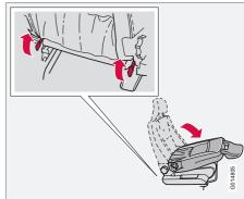
The front passenger's seat backrest can be folded down to provide room for long loads.
