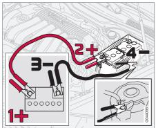
Follow these instructions to jump start your vehicle's dead battery or to jump start another vehicle's dead battery using your vehicle. If the 12-volt auxiliary battery to be used is in another vehicle, check that the vehicles are not touching to prevent premature completion of a circuit. Be sure to follow jump starting instructions provided for the other vehicle.
