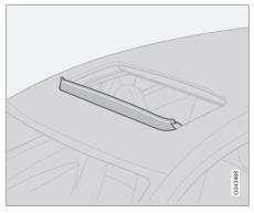
The moonroof is equipped with a wind blocker that folds up when the moonroof is open.
