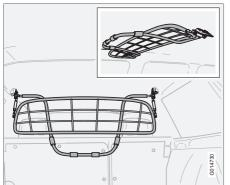
The steel grid prevents cargo from being thrown forward into the passenger area in the event of sudden braking.
