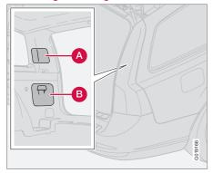
All bulbs in the taillight cluster can be replaced from the cargo area. To access the bulb holders:
