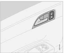
The switch near the door opening handle on the driver's door can be used to lock or unlock all doors and the tailgate, open the side windows<sup>1</sup>, and to set the alarm.
