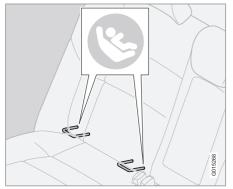
ISOFIX/LATCH lower child restraint anchors
