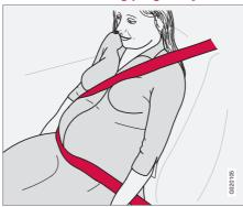
The seat belt should always be worn during pregnancy. But it is crucial that it be worn in the correct way. The diagonal section should wrap over the shoulder then be routed between the breasts and to the side of the belly. The lap section should lay flat over the thighs and as low as possible under the belly. It must never be allowed to ride upward. Remove all slack from the belt and insure that it fits close to the body without any twists.
