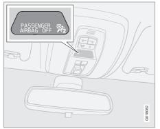
Occupant Weight Sensor (OWS) indicator light
