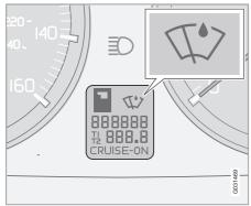
The rain sensor regulates windshield wiper speed according to the amount of water on the windshield. The sensitivity of the rain sensor is adjusted by moving the thumb wheel (C in the illustration on the previous page) up (the wipers will sweep the windshield more frequently) or down (the wipers will sweep the windshield less frequently).
