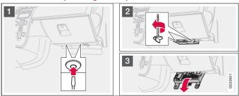
The fuse box in the passenger compartment is located under the glove compartment.
