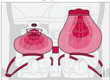
The front airbags supplement the three-point seat belts. For these airbags to provide the protection intended, seat belts must be worn at all times.
