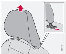
The front seat head restraints are designed so that they can be adjusted to two different height positions.
