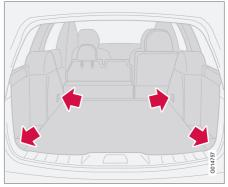
The eyelets in the cargo area can be used to fasten accessory load and lashing straps, load nets, and other load anchors.
