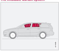
This system consists of inflatable curtains located along the sides of the roof liners, stretching from the center of both front side windows to the rear edge of the rear side door windows. It is designed to help protect the heads of the occupants of the front seats and the occupant of the outboard rear seating positions in certain side impact collisions.
