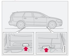
If a garage jack is used to lift the vehicle, the two jack attachments points should be used. They are specially reinforced to bear the weight of the vehicle. A garage jack can also be placed under the front of the engine support frame. Take care not to damage the splash guard under the engine. Ensure that the jack is positioned so that the vehicle cannot slide off it. Always use axle stands or similar structures.
