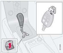
Shiftlock prevents the gear selector from being moved out of the **P** position unless the ignition key is in position **II** and the brake pedal is depressed.
