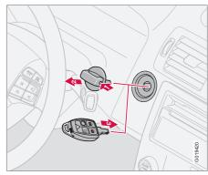
Removing the keyless drive start control
