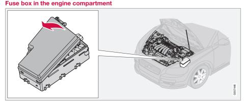
The fuse box in the engine compartment has positions for 36 fuses.
