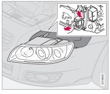
Disconnect the wiring connector by pressing down the clip with your thumb while at the same time pulling the connector with your other hand.
