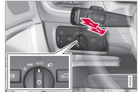
Stalk switch and knob for headlamp control.
