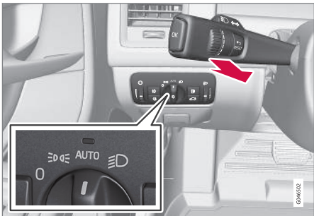
Stalk switch and knob for headlamp control in AUTO position.
