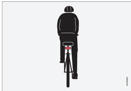
Optimum examples of what the system interprets as a cyclist - with clear body and bicycle con-
