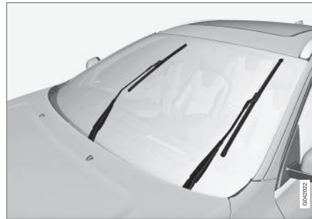
Wiper blades in service position.
