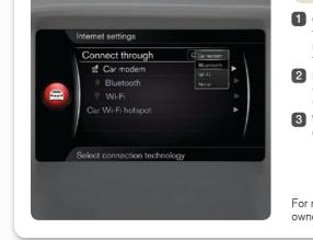
1 Connect the mobile phone via Bluetooth<sup>®</sup> or activate tethering in the phone for Wi-Fi connection. For car modem connection, fit the SIM card into the reader in the glovebox.
