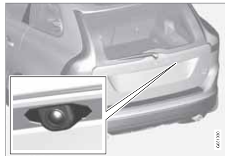
Camera location next to the opening handle.
