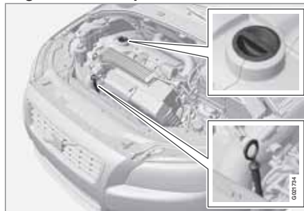
Dipstick and filler pipe.
