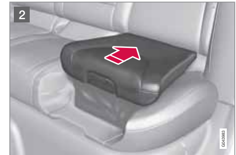
2 Press the booster cushion backwards to lock.
