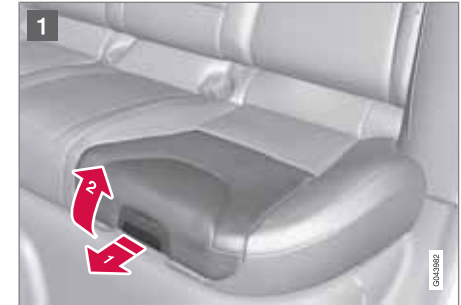
1 Pull the handle forward and up in order to release the booster cushion.
