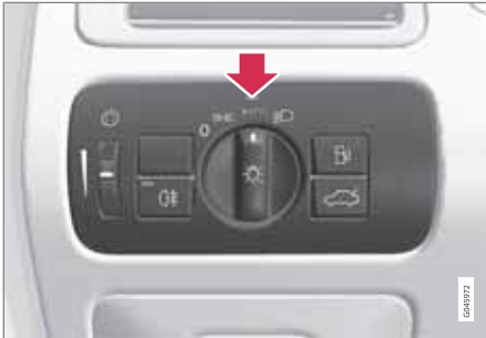
Light switch in position AUTO .
