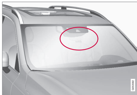
Radar unit location.
