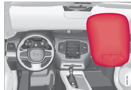
Front passenger airbag in front seat.
