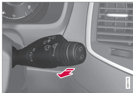
Washing function, right-hand stalk switch.
