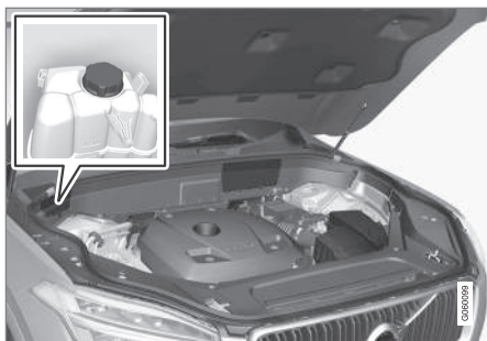
Coolant expansion tank.
