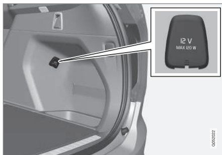
12 V electrical socket in cargo area*.
