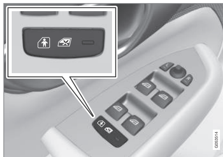
Button for electric activation and deactivation.
