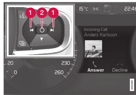
Message in the driver display 7 and the steering wheel's right-hand keypad.
