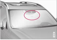
The area marked in the illustration must be kept free of decals, objects, solar film, etc.  $^{64}$
