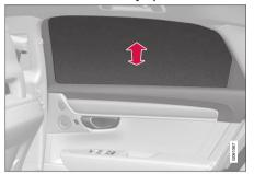
Each of the sun shades can be fully retracted or fully extended.
