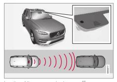
Location of the camera and radar sensor<sup>65</sup>.
