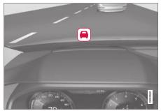
Collision warning symbol on the windshield<sup>67</sup>.
