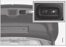
> The trunk lid will close automatically - the trunk lid will remain unlocked.
