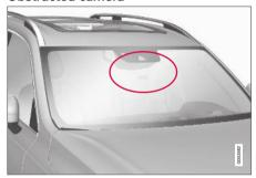
The area marked in the illustration must be kept free of decals, objects, solar film, etc.<sup>60</sup>
