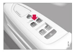
The panoramic roof and sun curtain can also be operated with the controls in the right-side rear door.
