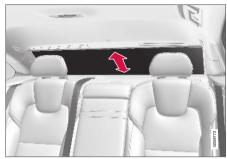
An electrically operated sun curtain is integrated in the rear window shelf.
