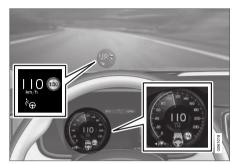
The previous illustration<sup>59</sup> shows that Pilot Assist is set to maintain a speed of 110 km/h (68 mph) and that there is no target vehicle ahead to follow.
