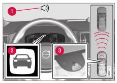
Collision warning audible signal and symbol<sup>35</sup>.
