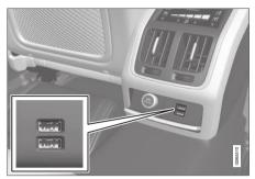
USB ports (type A) on rear of tunnel console for charging phones and tablets for example<sup>6</sup>.
