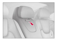
When the handle is rotated to its maximum position, the armrest is unlocked and can be folded down.
