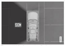
The vehicle's left-side camera is malfunctioning.
