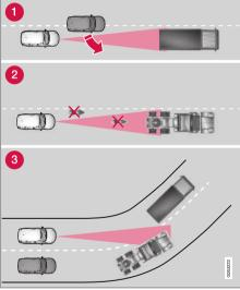
The radar sensor's field of vision.
