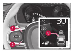
Controls for setting a time interval.
