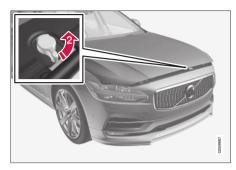
Turn the handle under the front edge of the hood counterclockwise to release the catch and lift the hood.
