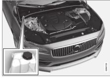
Coolant expansion tank, left-hand drive vehicle.
