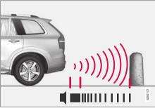
Continuous tone warning signal when the obstacle is less than approx. 30 cm (1 ft) from the vehicle <sup>107</sup>
