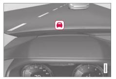
Collision warning symbol on the windshield<sup>36</sup>.
