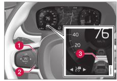
Controls for setting a time interval<sup>40</sup>.
