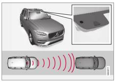
The camera/radar sensor measures the distance to the vehicle ahead<sup>34</sup>.
