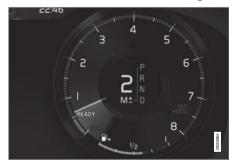
Manual shifting mode in the instrument panel<sup>2</sup>.
