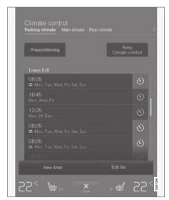
Parking climate functions are controlled from the **Parking climate** tab in the center display's Climate view.
