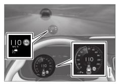
The previous illustration<sup>51</sup> shows that Adaptive Cruise Control is set to maintain a speed of 110 km/h (68 mph) and is following a target vehicle ahead, which is traveling at the same speed.
