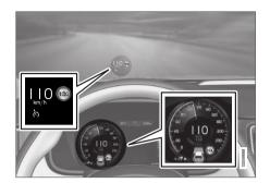
The previous illustration<sup>51</sup> shows that Adaptive Cruise Control is set to maintain a speed of 110 km/h (68 mph) and that there is no target vehicle ahead to follow.
