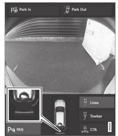
The screen can display colored sensor fields on the vehicle symbol<sup>115</sup>.
