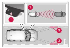
The camera/radar sensor monitors the distance to the vehicle ahead and detects lane markings<sup>52</sup>.
