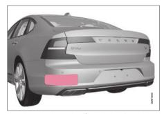
Keep the marked area clean (on both the left and right sides of the vehicle)  $^{83}$ .
