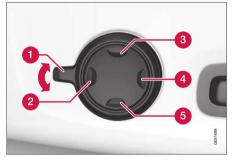
Activate the multifunction control by turning the control 1 upward/downward. The seat settings view will appear in the center display.
