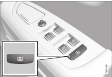
Briefly press the button - the sun curtain will automatically move to its end position, up or down.
