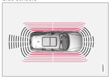
Rapid pulsing warning signal when the obstacle is less than approx. 25 cm (0.8 ft) from the vehicle <sup>107</sup>.
