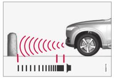
Continuous tone warning signal when the obstacle is less than approx. 30 cm (1 ft) from the vehicle <sup>107</sup>.
