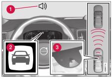
Collision warning audible signal and symbol<sup>53</sup>.
