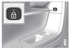
The indicator light in the button is on when the door is locked  $% \left\{ 1,2,\ldots ,n\right\}$
