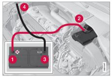
Connecting the jumper cables
