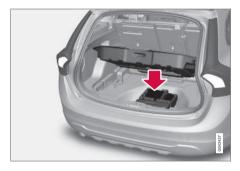
The jack\*, towing eyelet and tools\* are stowed under the floor of the cargo area.
