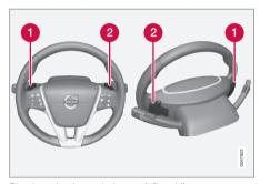
Steering-wheel mounted gear shift paddles
