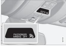
Occupant Weight Sensor (OWS) indicator light
