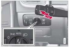
Headlight switch and steering wheel lever
