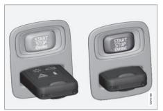
Ignition slot with remote key inserted (see Ignition modes (p. 82) for more information on ignition modes)
