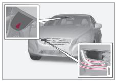
Camera and radar sensor<sup>8</sup>.
