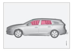
This system consists of inflatable curtains located along the sides of the roof liners, stretching from the center of both front side windows to the rear edge of the rear side door windows.
