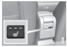
Heat control for the outboard seating positions is done in the same way as for the front seats.
