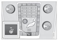
Button for steering wheel heating
