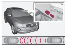
Location of the laser sensor in the windshield<sup>7</sup>
