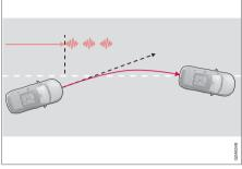
LKA provides vibrations in the steering wheel and steering assistance  $^{\!13}\!.$
