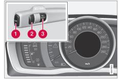
Analog Instrument panel and menu controls
