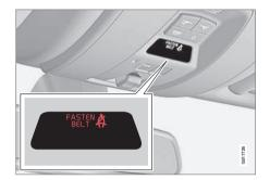
The audio reminder is speed dependent, and in some cases time dependent. The visual reminder is located in the roof console and in the combined instrument panel (p. 67).
