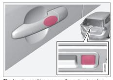
The touch-sensitive area on the outer door handles and the rubberised button next to the tailgate's rubberised pressure plate.
