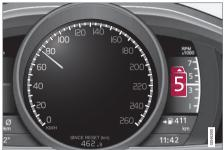
Combined instrument panel "Digital" with gear shift indicator.
