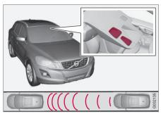
Laser sensor transmitter and receiver window14.
