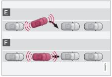
When the car has reversed into the parking space, it must be straightened up and stopped.
