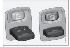
Ignition switch with remote control key extracted/inserted.
