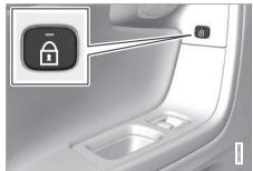
The button's lamp illuminates when the door is locked.
