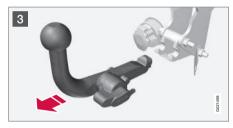
3 Turn the locking wheel down fully, until it comes to a stop. Hold it in this position while pulling the towbar rearward and upward.
