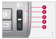
Thumbwheel positions for different load cases.
