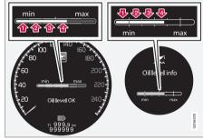
The figures 1-4 represent filling level. Do not fill more oil if filling level (3) or (4) is shown. Recommended filling level is 4. Message and graphic in the display. The left-hand display is shown in the digital combined instrument panel and the right-hand in the analogue.
