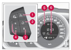
The steering wheel buttons and combined instrument panel in cars **with** speed limiter<sup>4</sup>.
