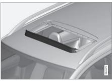
The sunroof has a wind deflector that is folded up when the sunroof is in the open position.
