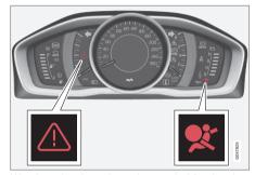
Warning triangle and warning symbol for the airbag system (p. 34) in the analogue combined instrument panel.
