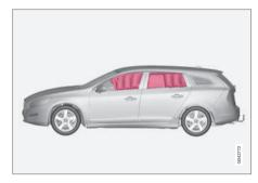
Inflatable curtain IC (Inflatable Curtain) is part of the SIPS system (p. 38) and the airbag system (p. 34). It is fitted along both sides of the headlining and helps protect the driver and passengers in the car's outer seats. A sufficiently violent collision trips the sensors and the inflatable curtain is inflated.
