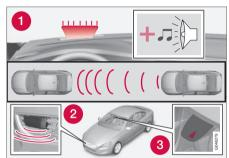
1. Collision warning system warning lamp and warning sound<sup>8</sup>.
