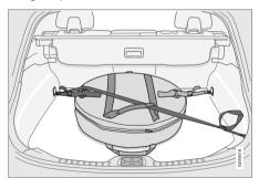
Cars with four load retaining eyelets.
