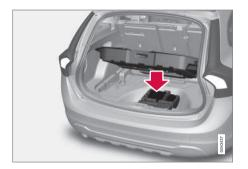
Located under the cargo area floor are the car's towing eye, jack\* and wheel wrench\*. There is also space here for the sleeve for the locking wheel bolts and tools for the plastic wheel bolt caps.
