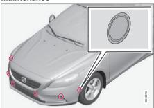
The PAP sensors are located in the bumpers<sup>34</sup> - 6 front and 4 rear.
