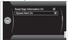
The driver can opt to receive a warning when the applicable speed limit is exceeded by 5 km/h (5 mph) or more. This warning is given by the symbol showing the applicable maximum speed temporarily flashing when this
