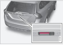
Rubber plate with electrical contact.
