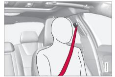
Correctly fitted seatbelt.
