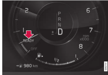
The function is active and the engine has auto-stopped.
