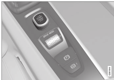
Start knob in the tunnel console.
