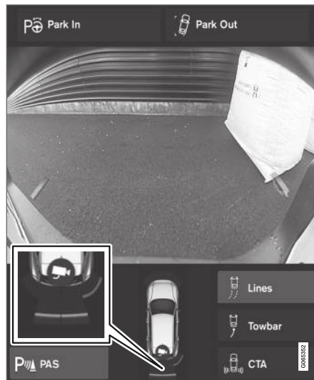
The screen can display colored sensor fields on the vehicle symbol 121 .
