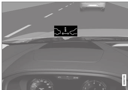
Distance Alert warning symbol on the windshield 36 .
