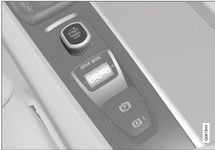
Start knob in the tunnel console.
