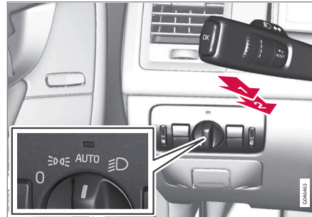
Stalk switch and knob for headlamp control.
