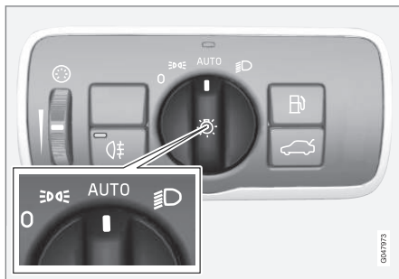
Knob for headlamp control in AUTO position.
