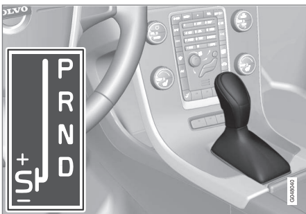
D: Automatic gear positions. +/-: Manual gear positions. S 8 : Sport mode*.
