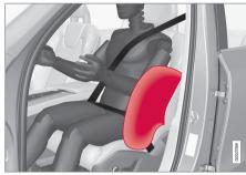
The side airbags are fitted in the outer backrest frames of the front seats and help to protect the driver and passengers in the front seat.
