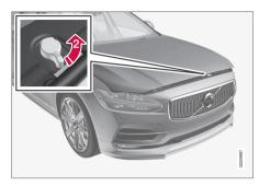
Yurn the handle under the bonnet anticlockwise to release the bonnet from the lock catches and lift the bonnet.
