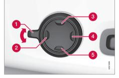
Activate the multi-function control by turning the control **1** upwards/downwards. The seat settings view will be shown in the centre display.
