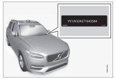
VIN is positioned in a similar place on all models.
