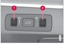
A car with LED<sup>2</sup> headlamps\* has automatic headlamp levelling and therefore does not have the thumbwheel for headlamp levelling.
