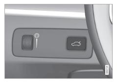
Long press on the instrument panel's button. Keep it depressed until the tailgate starts to open.
