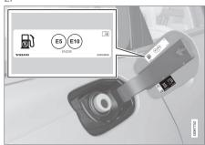
Choose fuel that is approved for use in the car in accordance with the identifier<sup>24</sup> on the inside of the fuel filler flap. See information on approved fuels and the identifier in the sections on "Petrol" and "Diesel" respectively.
