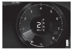
Driver display when changing gear with steering wheel paddles in manual gearshift mode, large gear lever.
