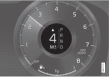
Gear shift indicator in 12-inch driver display for large gear lever\*.
