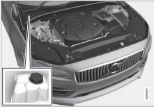
Coolant expansion tank, right-hand drive car.
