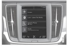
Many of the main functions of the car are controlled from the centre display, a touch screen which reacts to touch. The number of physical buttons and controls in the car is therefore minimal. The screen can even be operated while wearing gloves.
