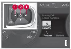
Examples of messages in the driver display<sup>6</sup> and the steering wheel's right-hand keypad. The figure is schematic - parts may vary depending on car model.
