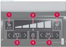
Controls for heated rear seat\*.
