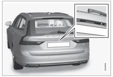
Rubberised pressure plate on the tailgate can only be used for unlocking.
