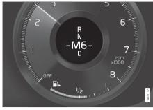
Overview of the shift pattern in the driver display for small gear lever.
