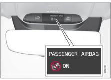
> A text message and a warning symbol in the roof console indicate that the airbag for the front passenger seat is activated.
