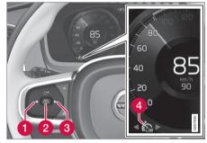
The speed limiter cannot be activated until after the engine has been started. The lowest maximum speed that can be stored is 30 km/h (20 mph).
