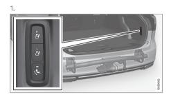
Open the tailgate. A button for extending/ retracting the towbar is located on the right-hand side at the rear of the cargo area. An indicator lamp in the button must illuminate with a constant orange glow for the extension function to be active.  Press and release the button – extension might not start if the button is pressed for too long.
