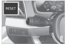
Reset all information in trip meter TM (i.e. mileage, average consumption, average speed and driving time) with a long press on the **RESET** button on the left-hand stalk switch.
