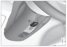
Lever for steering wheel adjustment.
