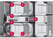
Location of adjustable air vents in the passenger compartment.
