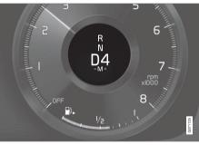
Driver display when changing gear with steering wheel paddles, small gear lever.
