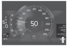
Examples of trip computer information in the 8-inch driver display. The figure is schematic - parts may vary depending on car model.
