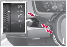
Steering wheel stalk switch with rotating ring.
