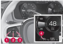
In order to start the cruise control from the standby mode, the car's current speed must be 30 km/h (20 mph) or higher.
