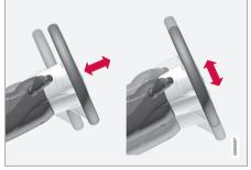
The steering wheel can be adjusted for height and for depth.
