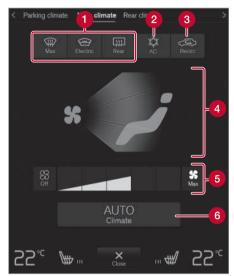
Max, Electric, Rear - Controls for defrosting the windows and door mirrors.
