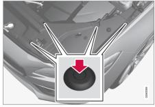
Press down the pins into the plastic cover's four clips using a screwdriver or similar and lift away the cover.
