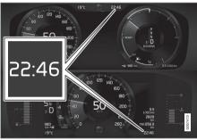
Clock location in the 12-inch<sup>\*</sup> and 8-inch driver display. The figure is schematic - parts may vary depending on car model.
