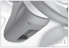
Lever for steering wheel adjustment.
