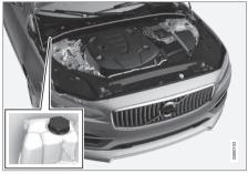
Coolant expansion tank, left-hand drive car.
