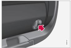
Detach the panel on the inside of the tailgate by first turning the two knobs a quarter turn anticlockwise and then unhooking the panel. Place the panel to one side.
