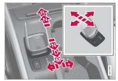
Overview of small gear lever and gear positions.
