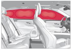
The inflatable curtain is mounted along both sides of the headlining and helps protect the driver and outer seat passengers of the car. The panels are labelled with **IC AIRBAG**.
