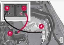
Attachment points for the jump leads. The appearance in the engine compartment may vary depending on car model and equipment level.
