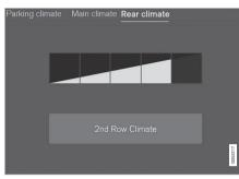
The fan control buttons in the tab **Rear climate** in the climate view.
