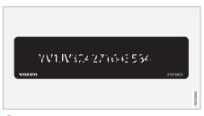
**7** Decal for the car's identification number - VIN (Vehicle Identification Number).
