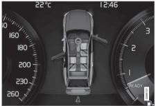
Graphics in the driver display with different types of warnings. The warning colour on the door and tail-gate is dependent on the vehicle's speed.
