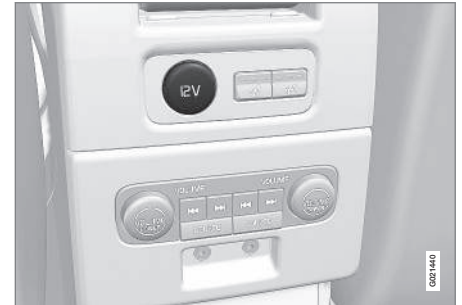
12 V socket in tunnel console, rear seat.
