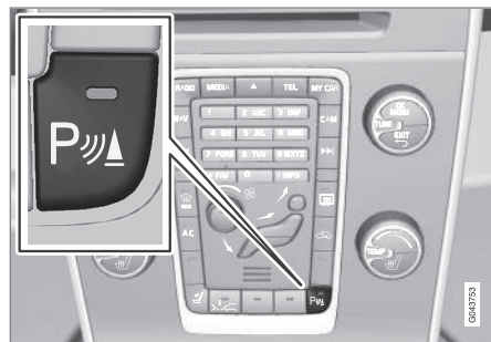
On/Off for parking assistance and CTA sensors.
