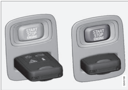
Ignition switch with remote control key extracted/inserted.
