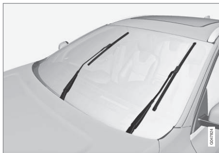
Wiper blades in service position.
