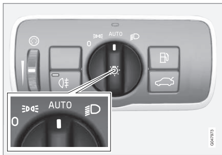
Knob for headlamp control in AUTO position.
