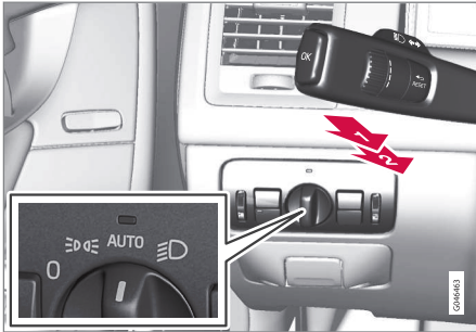
Stalk switch and knob for headlamp control.
