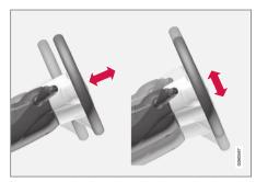
The steering wheel's reach and height can be adjusted.
