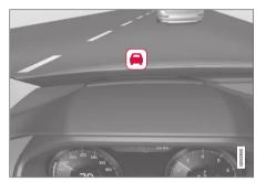
Collision warning symbol on the windshield<sup>39</sup>.
