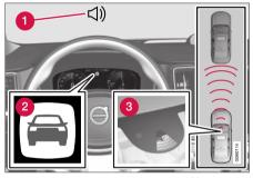
Collision warning audible signal and symbol<sup>56</sup>.
