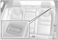
Buttons for folding down the seats, located on the top section of the left-side rear seat.
