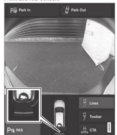
The screen can display colored sensor fields on the vehicle symbol  $^{121}$ .
