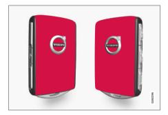
For a Red Key, it is possible to define the vehicle's maximum speed, set speed reminders and limit the audio system's volume. Several of the driver support systems will also always be active. Otherwise, the Red Key functions in the same way as a standard remote key.
