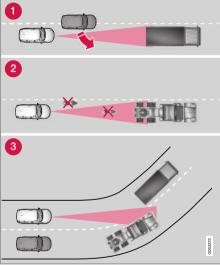
The radar sensor's field of vision.
