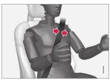
The belt should be positioned closely over the shoulder (against the collarbone, not down over the arm).
