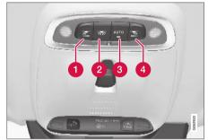
The controls in the ceiling console for the front reading lights and courtesy lighting.
