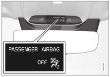
Occupant Weight Sensor (OWS) indicator light
