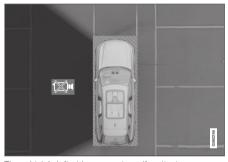
The vehicle's left-side camera is malfunctioning.
