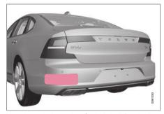
Keep the marked area clean (on both the left and right sides of the vehicle)<sup>86</sup>.
