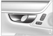
Alternative unlocking method using side door opening handle  $^{\rm 14}.$
