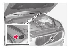
Fill washer fluid into the reservoir with the blue cover. The reservoir is used for both the windshield washer and the headlight washer\*
