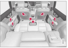
Storage compartment in the door panel and storage pocket\* in the front seat backrest.
