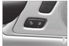
Button with indicator light for locking and unlocking in front door.
