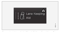
A warning triangle in the right-hand section of the button indicates that something is not working correctly.
