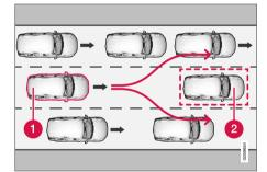
Your vehicle (1) cannot detect any potential escape routes for veering away from the vehicle ahead (2) and may therefore apply the brakes at an earlier stage.
