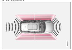
Rapid pulsing warning signal when the obstacle is less than approx. 25 cm (0.8 ft) from the vehicle <sup>113</sup>.
