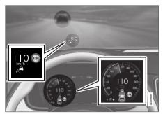
The previous illustration<sup>54</sup> shows that Adaptive Cruise Control is set to maintain a speed of 110 km/h (68 mph) and is following a target vehicle ahead, which is traveling at the same speed.
