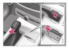
If the vehicle cannot be driven (e.g. due to a discharged battery), the gear selector must be moved to the  ${\bf N}$  position so that the vehicle can be moved.
