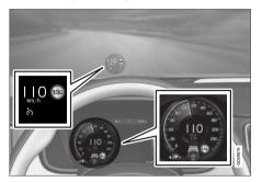
The previous illustration 62 shows that Pilot Assist is set to maintain a speed of 110 km/h (68 mph) and that there is no target vehicle ahead to follow.
