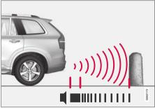
Continuous tone warning signal when the obstacle is less than approx. 30 cm (1 ft) from the vehicle <sup>113</sup>
