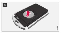
The battery's positive side (+) faces upward. Carefully pry out the battery as shown in the illustration.
