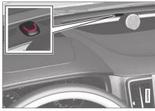
The locks and alarm indicator on the dashboard will display the status of the locking system.
