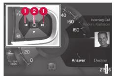
Messages in the instrument panel<sup>6</sup> and the right-side steering wheel keypad.
