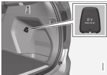
12 V electrical socket in cargo area*.
