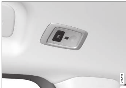
In cars with panorama roof* there are two lamp units, one on each side of the roof. 10
