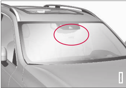
Location of the camera unit.
