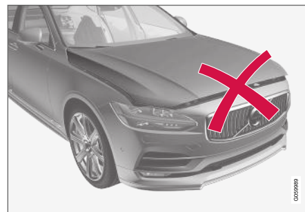
Bonnet not completely closed.
