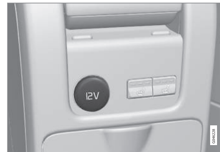
12 V socket in tunnel console, rear seat.
