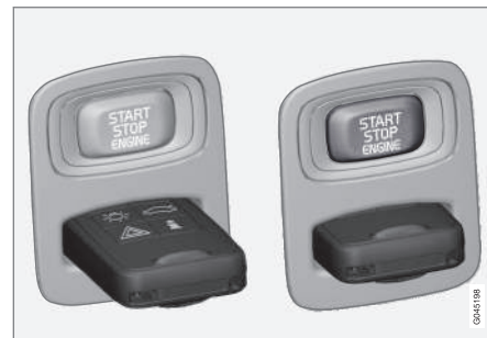
Ignition switch with remote control key extracted/inserted.
