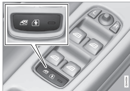
Control panel driver's door.
