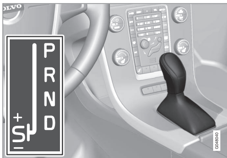
D: Automatic gear positions. +/-: Manual gear positions. S 5 : Sport mode*.
