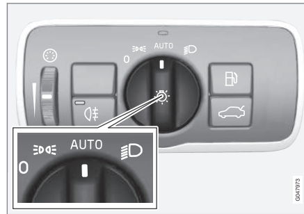
Knob for headlamp control in AUTO position.
