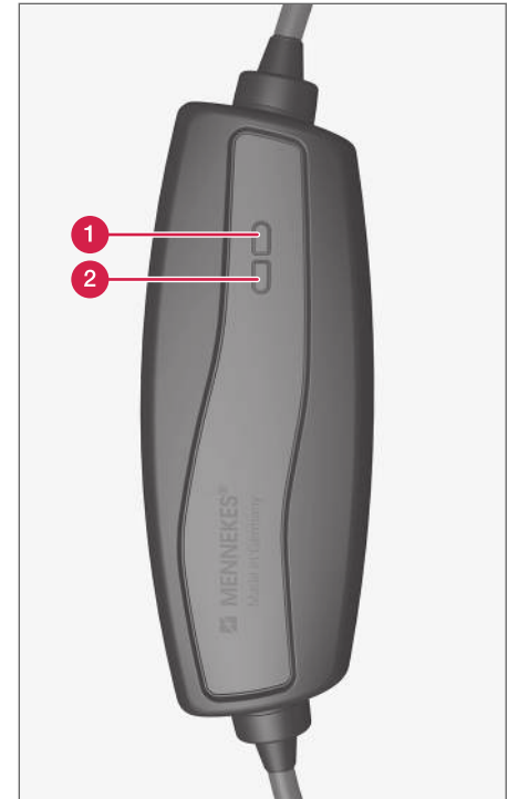
Control unit LED 9 lamps.
