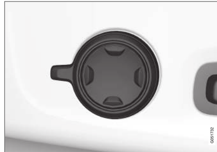
Multi-function control, located on the side of the seat's seating section.
