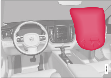
Front passenger airbag in front seat.
