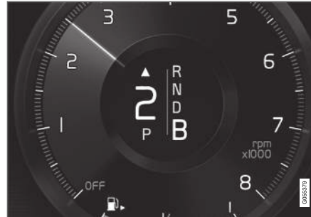
Gear shift indicator in the driver display 5 .
