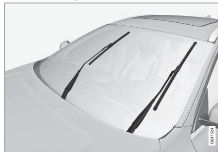
Viskerblade i servicestilling.
