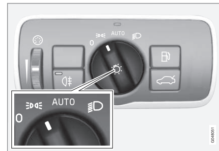
Lyspanelets knap i positionen for positions-/parkeringslys.
