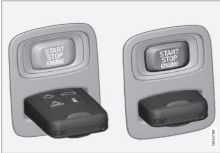
Ignition switch with remote control key extracted/inserted.
