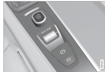
Start knob in the tunnel console.
