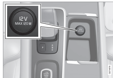
The tunnel console's front electrical socket for cars without wireless phone charger*.
