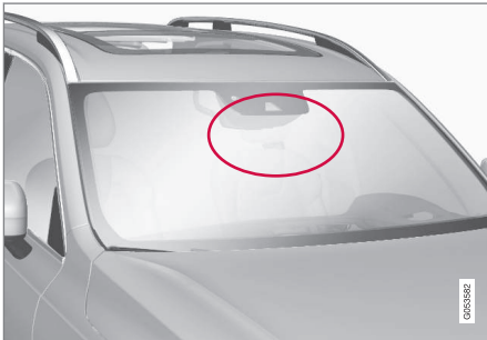
Radar unit location
