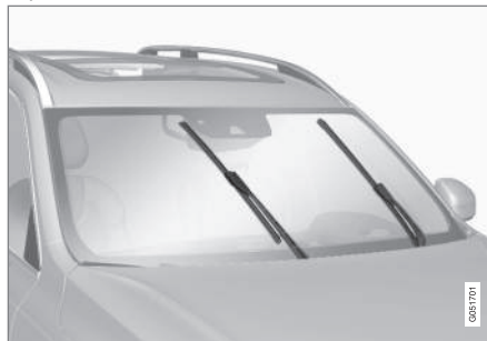
Wiper blades in service position.
