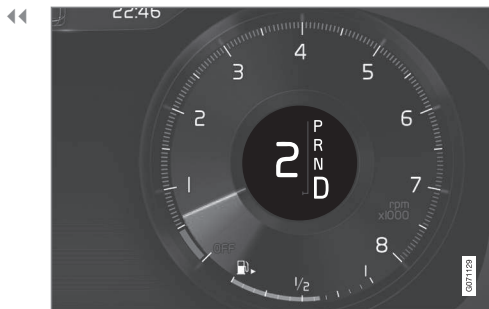
Driver display when changing gear with steering wheel paddles, large gear lever.
