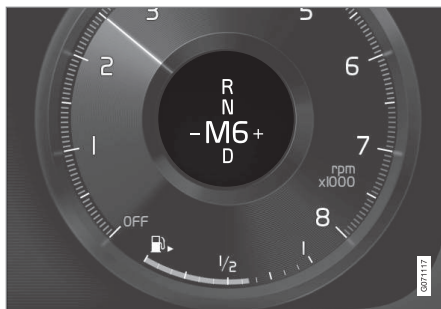
Overview of the shift pattern in the driver display for small gear lever.
