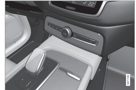
Overview of the small gear lever where it is not possible to deactivate the gear selector inhibitor.
