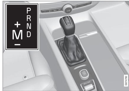
Overview of large gear selector and gear shift pattern in the instrument panel.
