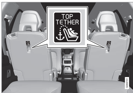
Six-seat models: Top tether anchors and symbols on the rear side of the second row backrests.
