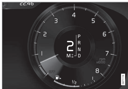
Overview of gear shift pattern in the instrument panel for large gear selector.
