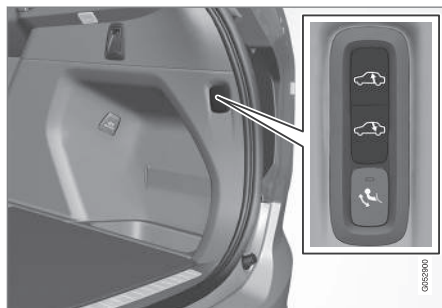
Controls for raising/lowering the car's rear section.
