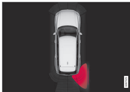
Illuminated icon for Cross Traffic Alert in the Park Assist System graphic on the screen.
