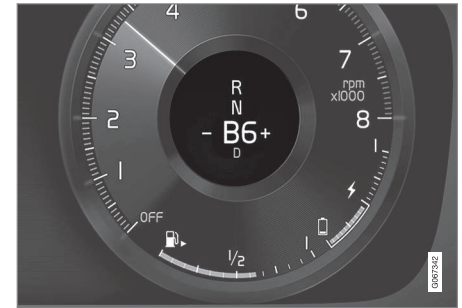
Gear shift indicator in the driver display 5 .
