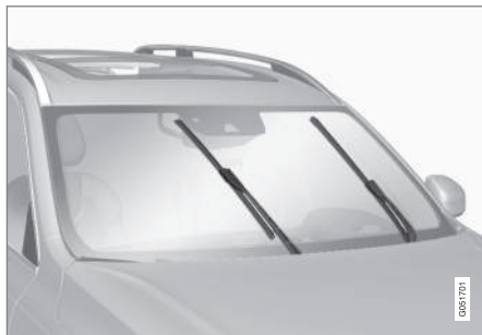
Viskerblade i servicestilling.
