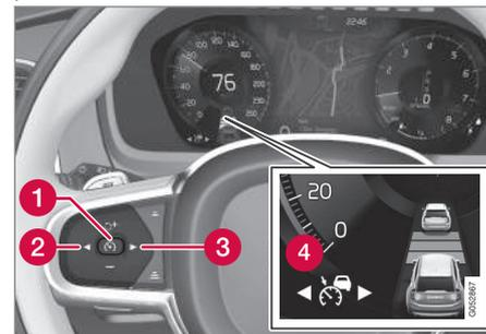
1. Appuyez sur la commande au volant
